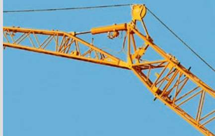
Adjustable folding jib (0° to 45°)
