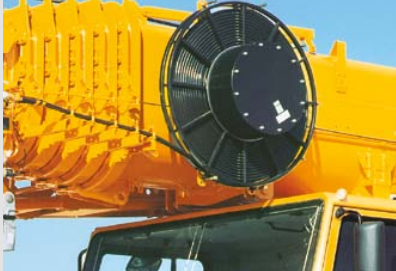
Hose reel for the hydraulic cylinder
