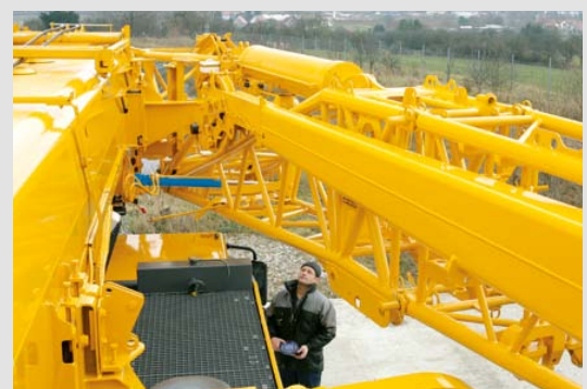
Hydraulic assistance for assembly of the swing-away jib with BTT
