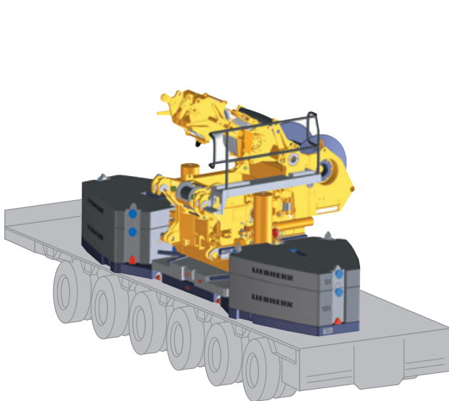
60 t-package with winch 3
